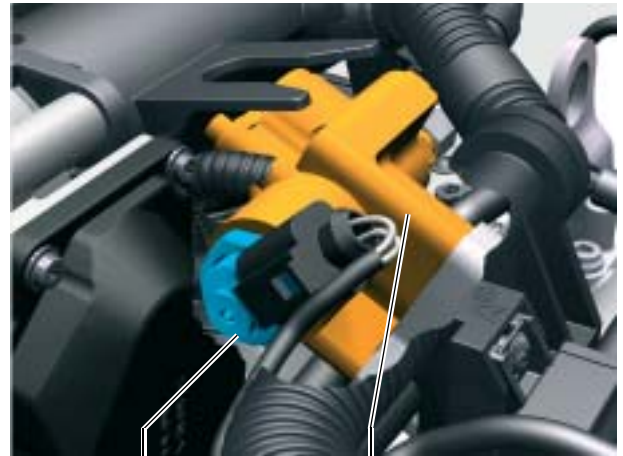
Fuel pressure regulating valve N276
