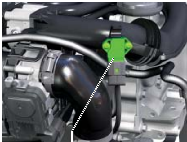
Intake manifold pressure sender G583 with intake air temperature sender G520
