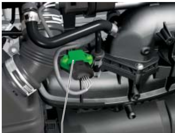
Intake manifold pressure sender G71 with intake air temperature sender G42
