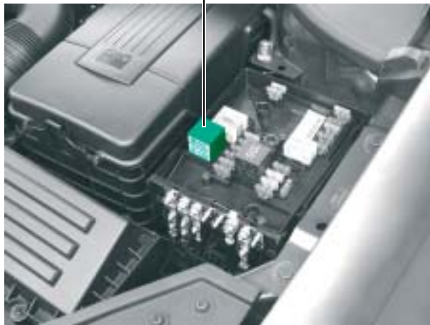
Sensor for current measurement G582
