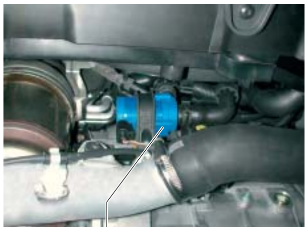
Coolant circulation pump V50
