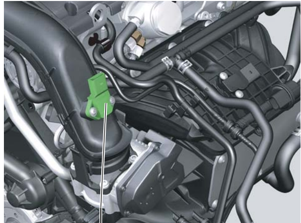
Charge air pressure sender G31 with intake air temperature sender G299 S405_042
