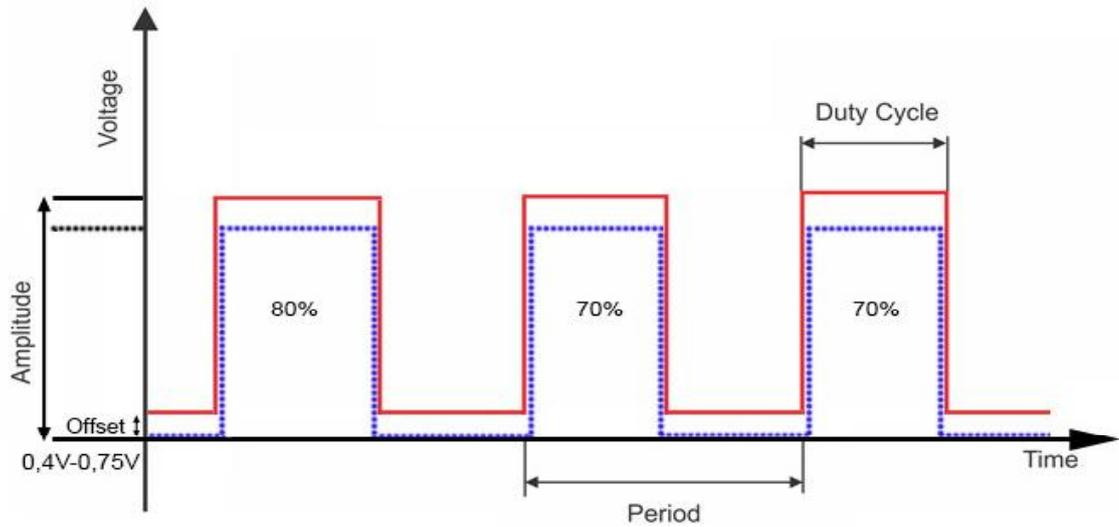
If the off-set were to exceed 0,75V, the ECU probably won't recognize the signal and because of that could calculate the wrong load of the alternator at that specific time.
