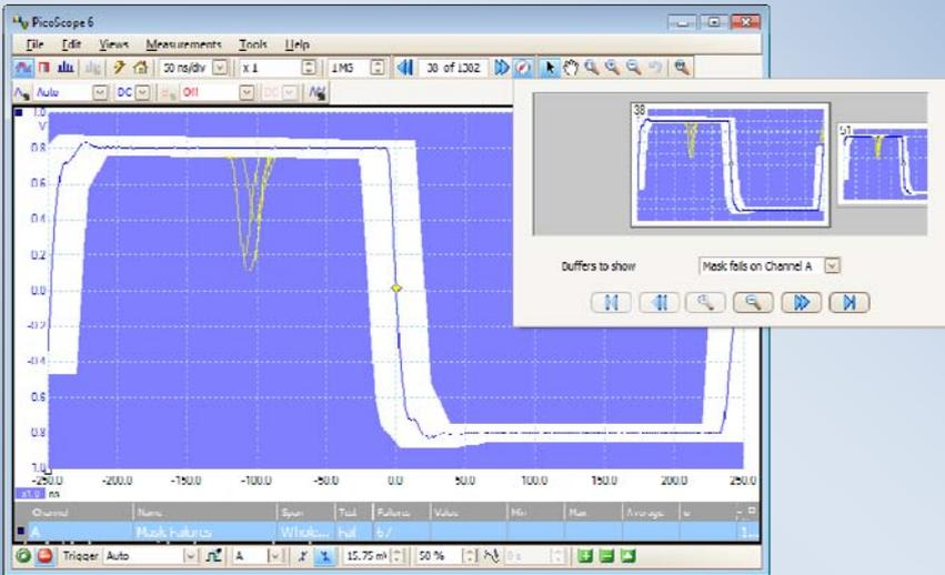
In the example above, we created a mask (the blue areas) around a good waveform using the **Tools > Masks** command and then the **Generate** button. This created a mask with the specified clearances around the waveform. We then set the Buffer Overview filter to "Mask fail on Channel A". This hid all of the 10,000 waveforms except the 100 or so that contained the glitch.
