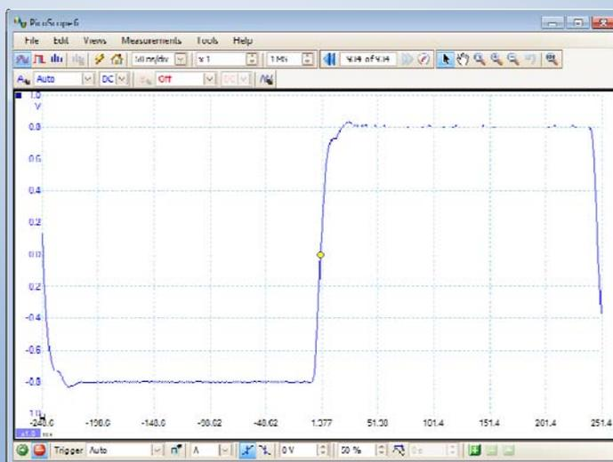
The above example shows that, even with PicoScope's optimized 20 Hz display update rate, only a tiny proportion of the input signal ever appears on the display. This makes it unlikely that you will spot an infrequent glitch. In some cases you can set up an advanced trigger to isolate the glitch, but this is possible only if you know what kind of signal you are looking for.
