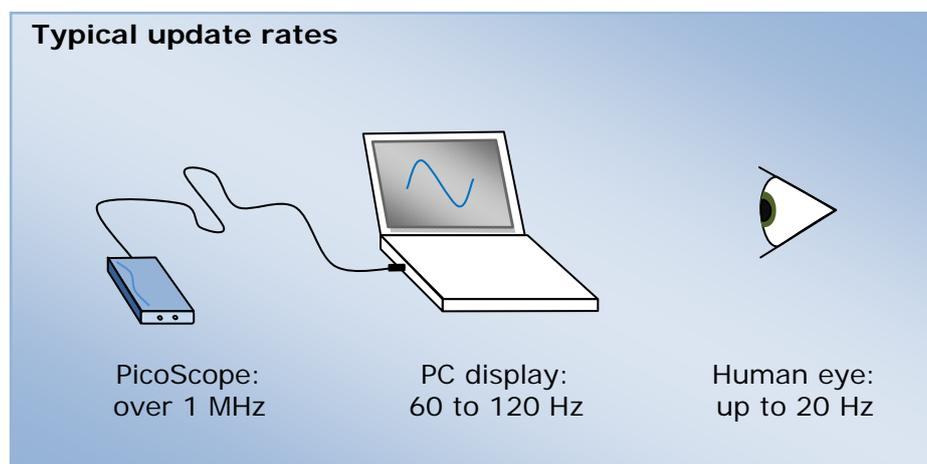
The data acquisition hardware can often capture millions of waveforms per second. Clearly, the digital oscilloscope needs to reduce the amount of captured data before displaying it, but how can it do this without throwing away important information? The answer is: it's up to you, the user. If you understand how to use the scope to filter out unwanted data, you will be able to search more efficiently for intermittent events like glitches.
