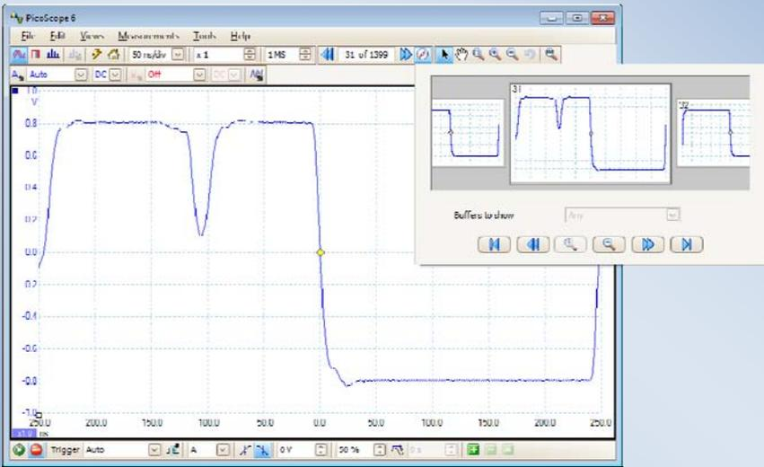
In the above example, the scope captured a closely spaced sequence of waveforms. By scrolling through the Buffer Overview, we found an example of the glitch. Selecting this waveform copied it to the main display, where a range of measurement tools such as vertical and horizontal rulers are available. We could also estimate the frequency with which the glitch occurs by counting the number of instances in the buffer.
