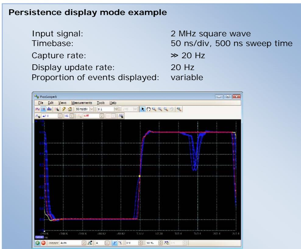
The hottest colors (such as red) indicate the densest areas of data where the majority of the waveforms are located. The coolest colors (such as blue) indicate transient events such as glitches and jitter.
