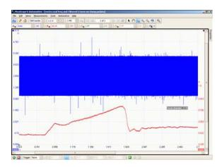
The blue trace shows the frequency output and the red shows the current drawn. The change in current drawn is only a few mA so it stretches the limits of what can be measured with the 60 A current clamp, even when set to the 20 A range.
