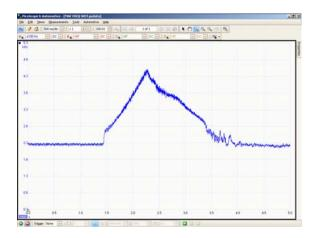
There are a few points to note. Firstly this option is only available on the PicoScope 4000 range of automotive scopes, as it requires hardware resources not available in earlier products. Secondly, in PicoScope 6.4.28, the frequency measurement is a bit sensitive to noise. This will be addressed in future releases. Frequency measurement is enabled from the AC/DC drop-down menu.
