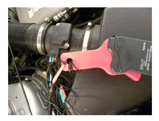
This "amplifies" the current 5 times so, although the scale shows 1 A, the actual range is 200 mA. We also switched on the low-pass filter to further clean up the signal.
