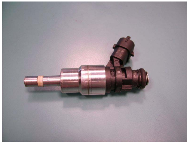
Figure 32. Bosch GDI single-hole injector
