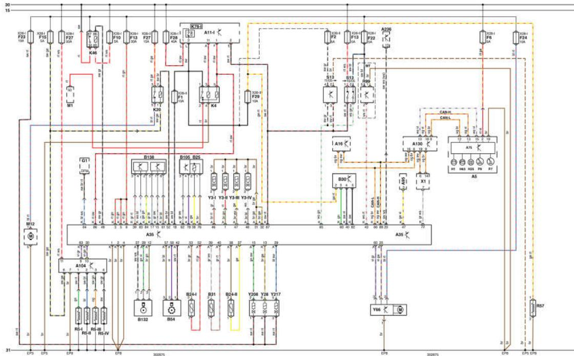
NOTE: In certain diagrams (Citroen, Peugeot & Renault), colour codes are replaced by numbers which are used to identify a particular cable and not the colour. In this instance, the cables will be numbered at each end close to the harness connector.
