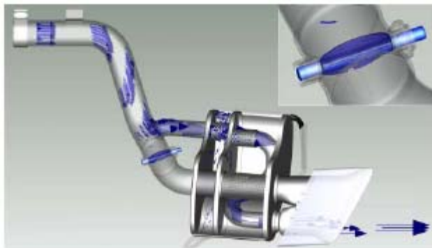
BY-PASS VALVE CLOSED
