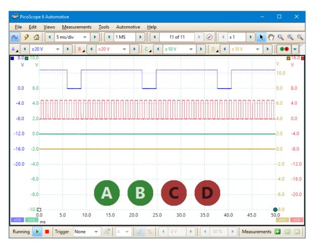
Every channel input on the PicoScope 4225 and 4425 scopes has an LED next to it. When ConnectDetect is activated for a channel, the LED for that channel is either green, to indicate that the test probe is directly connected across a component, or red to indicate that it is not. You can select which channels ConnectDetect is activated for
