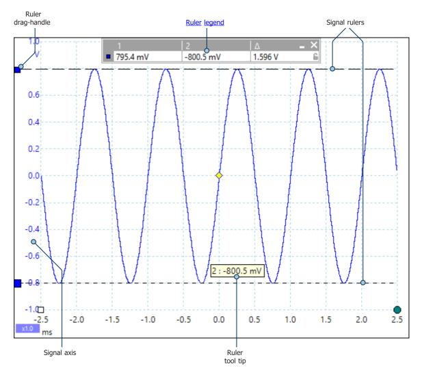
In the <u>scope view</u> above, the two colored squares to the left of the vertical axis are the ruler drag-handles for Channel A. Drag one of these downwards from its resting position in the top left corner, and a signal ruler (a horizontal dashed line) will extend from it.
