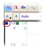
3. Drag the ruler handle downwards. A <u>signal ruler</u> (horizontal broken line) will appear across the view. Release the ruler handle when the ruler is where you want it.
