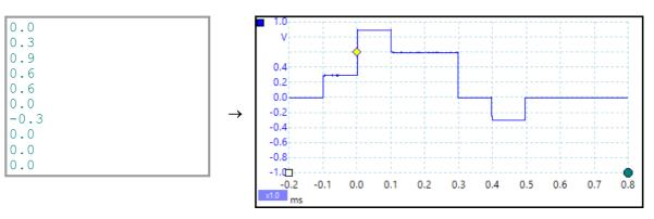
The minimum number of values a file may have is 10; the maximum is determined by the size of the AWG buffer (specified in the data sheet for your scope device).
