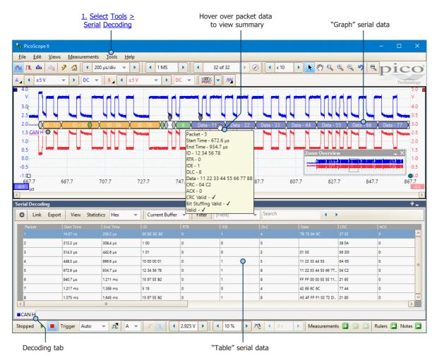
To start decoding your data, click **Tools** > **Serial Decoding** from the Menu bar. There are many <u>different protocols</u> available, and the data can be viewed in **Graph** or **Table** formats, or both. You can simultaneously decode multiple channels in different formats, and switch between them using the **Decoding tabs**.
