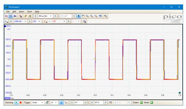
The colors indicate the frequency of the data. Red is used for the highest-frequency data, with yellow for intermediate frequencies and blue for the least frequent data. In the example above, the waveform spends most of its time in the red region, but noise causes it to wander occasionally into the blue and yellow regions. These are the default colors, but you can change them using the <u>Colors page</u> of the <u>Preferences</u> <u>dialog</u>.
