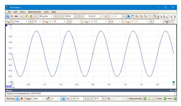
You can place a **Notes** area at the bottom of the PicoScope window, and you can enter any text you wish in it or paste text into it from other programs. This text is included when you save the waveform as a file.
