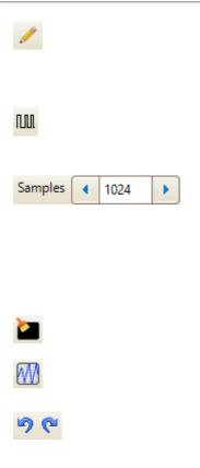
**Line Drawing mode.** Enters straight line mode, in which you can click on the waveform to draw a straight line from the previous point. To start a new series of lines, click the button again.
