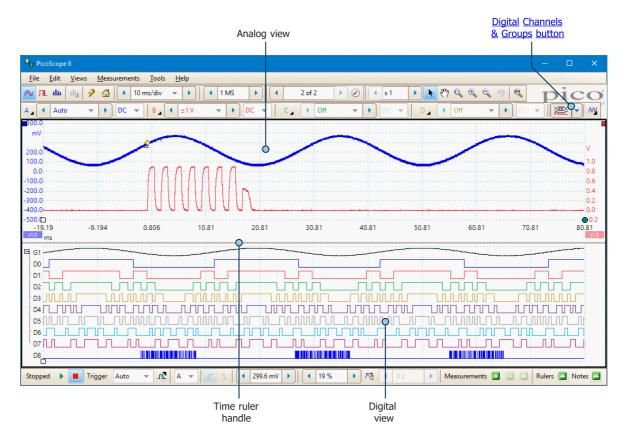
The **MSO view** shows mixed analog and digital data on the same horizontal scale.
