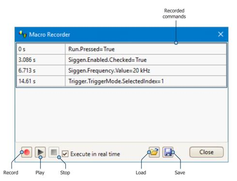
**Execute in real** Play back the macro at the same speed as it was recorded. When this box is not checked, playback will be as fast as possible.
