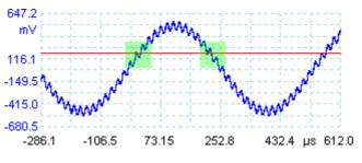
Noisy signal with a single threshold
