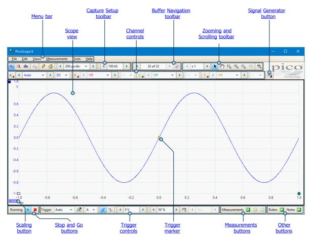
Note: additional buttons may appear in the main PicoScope window depending on the capabilities of the oscilloscope that is connected, and on the settings applied to the PicoScope program.
