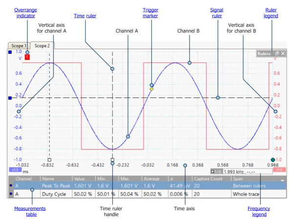
Scope views are available regardless of which mode - <u>scope mode</u> or <u>spectrum mode</u> - is active.
