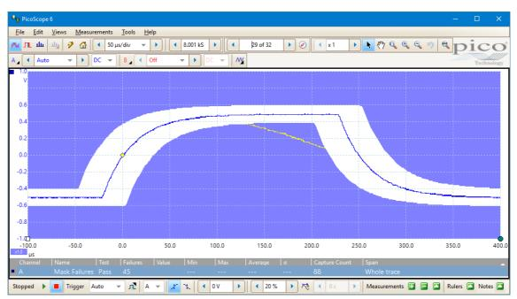
You now have a functioning mask limit test. Please refer to <u>Mask limit testing</u> for information on editing, importing and exporting masks. It is also possible to set up a mask limit test on a <u>spectrum</u> or <u>XY</u> view.
