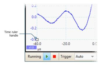
2. Drag the time ruler handle to the right. A <u>time ruler</u> (vertical broken line) will appear on the scope view. Release the ruler handle when the ruler is at the time you wish to use as the reference.
