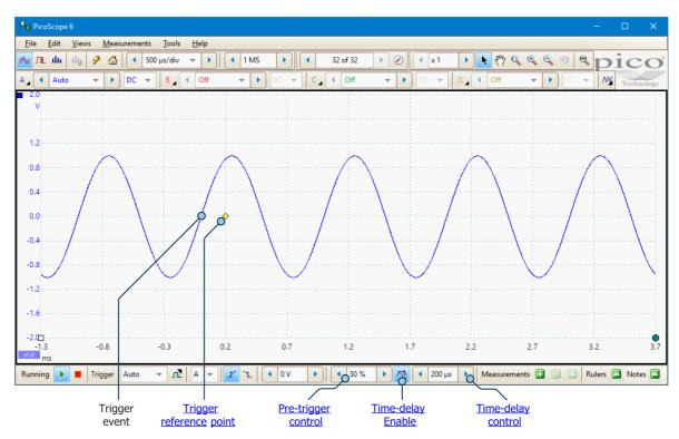
The **pre-trigger** control positions the scope view in relation to the **trigger reference point**, allowing you to decide how much of the waveform should appear before the reference point, and how much after it. In this example, it is set to 30%, so the trigger reference point appears 30% of the way across the display from the left-hand edge.
