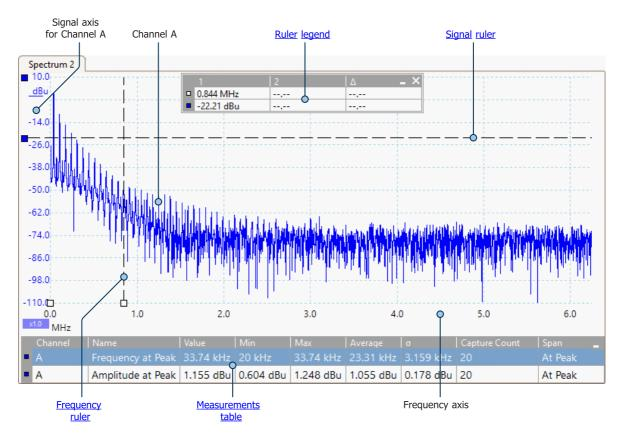
Spectrum views are available regardless of which mode - <u>Scope Mode</u> or <u>Spectrum</u> <u>Mode</u> - is active.
