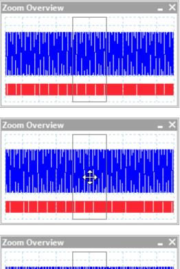
The **Zoom Overview** shows the full waveforms on all enabled channels. The rectangle indicates the area that is visible in the current view.
