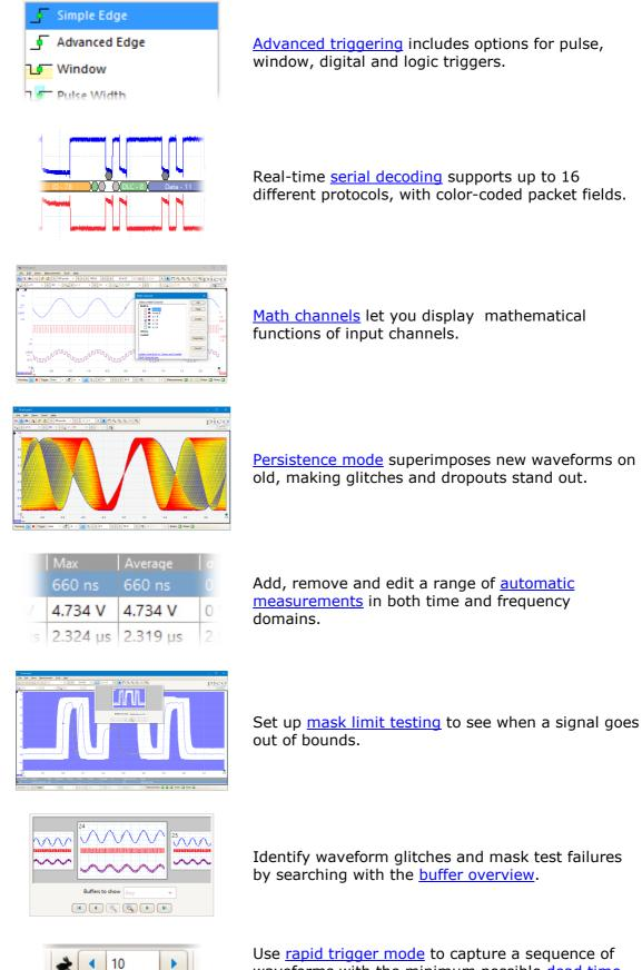
Use <u>rapid trigger mode</u> to capture a sequence of waveforms with the minimum possible dead time.
