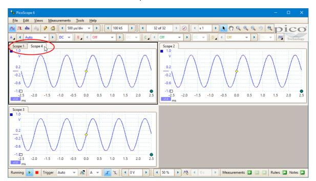
3. Release the mouse button. The Scope 4 view will move to its new location.
