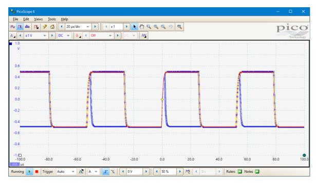
• Looking more closely, we can also see that there appears to be a much narrower pulse than usual immediately after the trigger marker. It is also visible approximately 50  $\mu$ s before the trigger marker and about 55  $\mu$ s later. Below is a close-up of one of these spikes:
