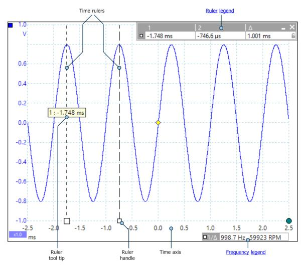
In the <u>scope view</u> above, the two white squares on the time axis are the **time ruler handles**. When you drag these to the right from the bottom left corner, the **time rulers** appear. The rulers work in the same way on a <u>spectrum view</u>, but the **ruler legend** shows their horizontal positions in units of frequency rather than time.
