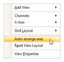
PicoScope automatically scales and offsets the channels to make them fit on the view without overlapping. This is the quickest way to tidy up the scope view:
