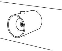
Input signal BNC connector on front of unit
