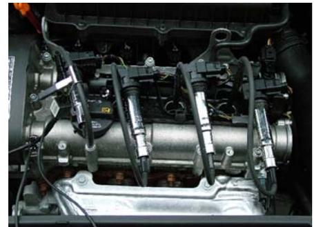
1. With the ignition turned off, disconnect the coil from the spark plug. This will inevitably require the multi-plug to be disconnected and reconnected. To aid this operation it may be worth spraying the plug with some release oil to prevent any damage to the release tabs.
