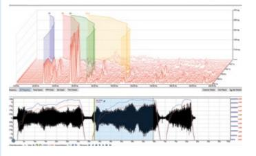
Our NVH kits use a combination of accelerometers, microphones and technical data to measure, calculate and analyze the rotating and vibrating components in a vehicle. By being able to correctly analyze the results you see on-screen, you can identify the root cause of your NVH issue.
