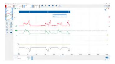
You can now explore the operation of the whole system with one capture. In the waveform shown below you can see the performance of the hydraulic system on a telehandler using the optional 300 litre/min Webtec flowmeter.
