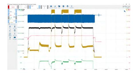
There is a huge amount of diagnostic information in this capture, showing both the basic operation of the system, as well as some of the feedback controls built into this vehicle. Engine speed can be inferred directly from the crank speed sensor by using a measurement, or as shown above, using a math channel.
